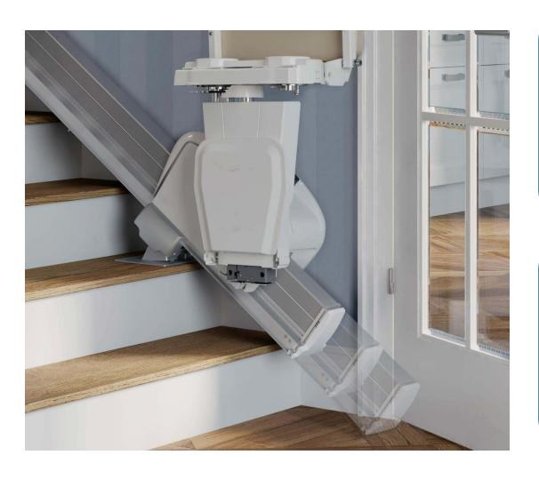
A Slide Track is slightly shorter than the length of your staircase. As you start to travel up the staircase the track will move with you. The track will reach the top of your stairs before the stairlift, it will then stop whilst your stairlift continues on its journey to the top where you can safely dismount. When you come downstairs the track will travel down with you so you can dismount safely at the bottom.
