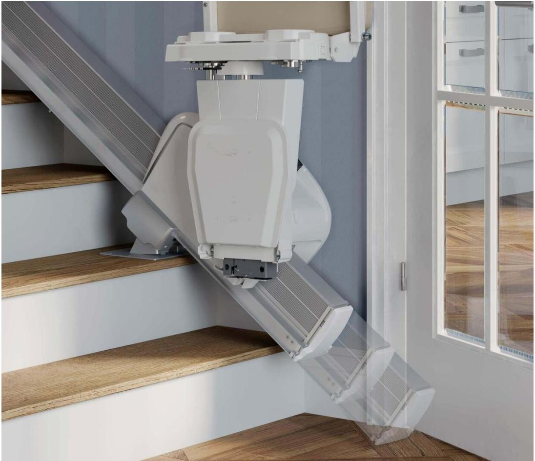
A Slide Track is slightly shorter than the length of your staircase. As you start to travel up the staircase the track will move with you. The track will reach the top of your stairs before the stairlift, it will then stop whilst your stairlift continues on its journey to the top where you can safely dismount. When you come downstairs the track will travel down with you so you can dismount safely at the bottom.
